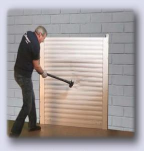
In impact testing, Qompact withstood 82 punches, 5 kicks, and 80 hits with a sledge hammer. The foam-filled shutter was destroyed in seconds.
